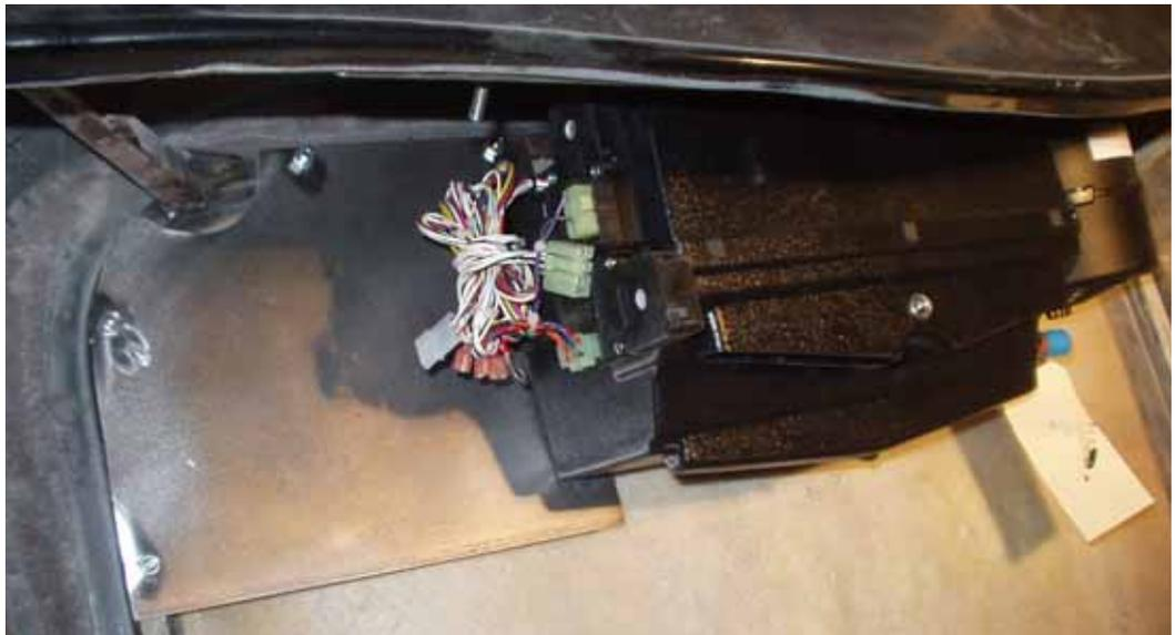
The condenser unit needs to be secured in the front to hold it away from the firewall and from moving around. The control unit needs to be mounted under the square tube, near the clamp.
