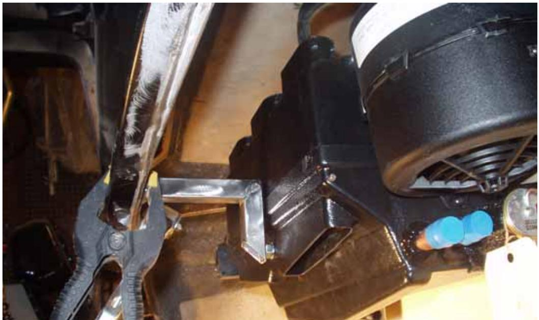
The body reveal tapered to the frame. Not exactly how I wanted it to be.....so I fixed it. Mixed some resin and viscofil to make the resin into a stiff paste. Some taped covered masonite to form the go and voila, it's pretty close. A little fiberglass on the inside and we're almost ready for the new old firewall.
