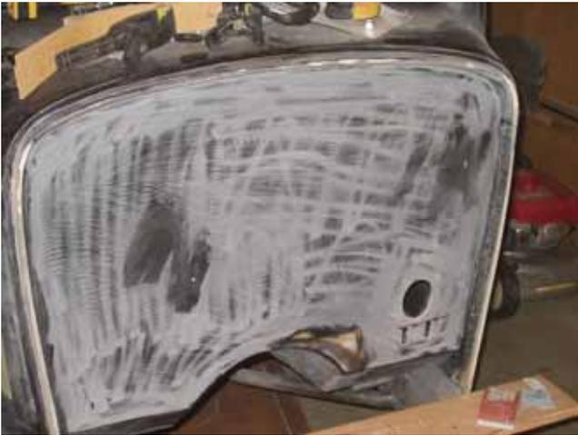
So the integral firewall gets roughed up and new, old, is laid over the resin glue concoction so that it doesn't rattle under hard acceleration. The bracing ensures full contact.
