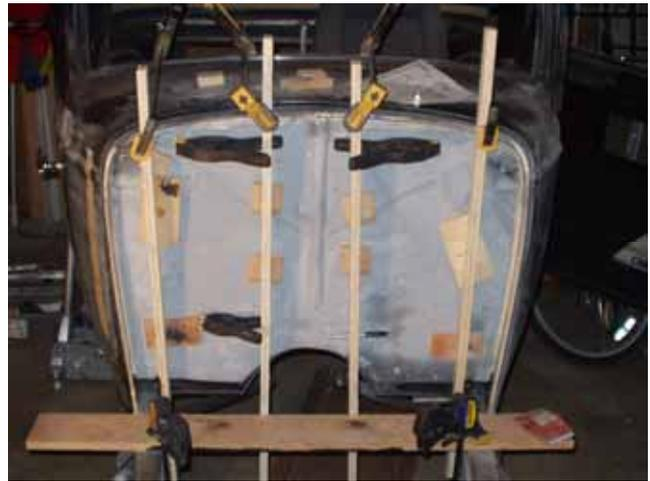
Voila. The finished new old firewall is in place. With some finishing around the edges, it will look like it's supposed to be there. Cut the steering column and clutch and brake pedal holes and we're good.
