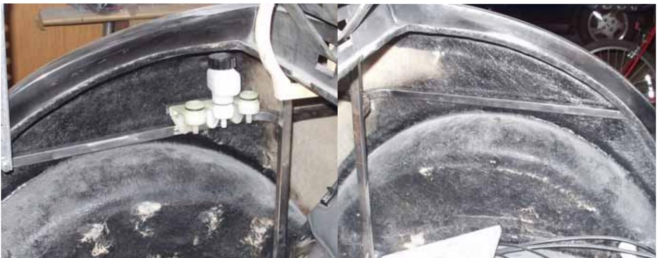
The pedals are taking some planning. Need to determine the correct size of the pedal pad, pad attachment to the arm which runs through the floor, so I could remove without taking part of the floor or a panel out. The pedal pads need to clear the steering column, symmetrical to the column and leave some room to put my left foot. No room for a dead pedal here!
